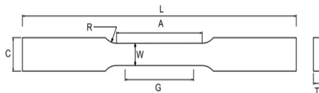
Figure 1: ASTM E8 standard test specimen
