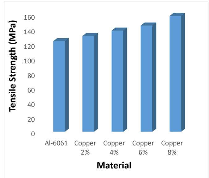
Figure 4: Variation of tensile strength of aluminum alloy 8011 by variation of copper concentration.
